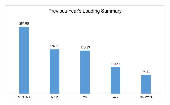
The Non-Coincident Peak Demand is 175.28 MW, which represents approximately 66.27% of the total substation capacity of 264.96 MVA at a power factor of 97.81%. The load factor, defined as the ratio between the Average Load of 105.44 MW and the Non-Coincident Peak Demand, is 60.06%. A reasonable estimate of the true minimum load is the fifth percentile load of 74.41 MW, which accounts for 42.38% of the Non-Coincident Peak Demand. Please refer to Annex "F" and Annex "F-1" for further details.
