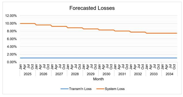
Transmission Loss is assumed to be at average of 1.08% while Distribution System Loss is expected to reach 9.97% by end Year 2025 and target to be reduced to 7.46% by Year 2034 (see Annex "I" for details).
